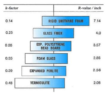
**Conductivity & Resistance of Insulating Materials:** With the lowest K-factor (conductivity) and highest R-value (resistance), urethane foam can provide more thermal resistance with less material than any other insulation.
