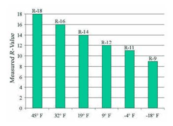
R-Value vs. Temperature: "There is a problem with loose-fill fiberglass attic insulation is cold climates. It appears that, as attic temperature drops below a certain point, air begins to circulate into and within the insulation, forming "convective loops" that increase heat loss and decrease the effective R-value. At very cold temperatures (-20F), the R-value may decrease by up to 50%."
